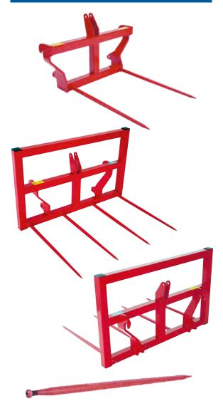
Double or quadruple bale spikes, with **Euro- and three-point bracket**, high-quality (square shaft) spring steel spikes 1,100 mm long (screw thread M  $22 \times 1.5$ ), thick-walled tube with welded tapered sleeves.
