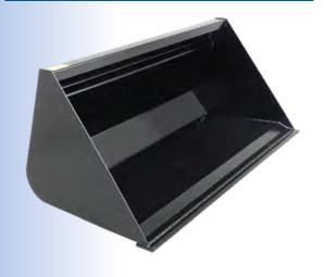
With LP-bracket for front-, telescopic- or wheel loaders (please order adapter plates separately), conical design for better sliding of the bulk material, hardened 500 HB cutting edge and protective runners at the bucket base.
