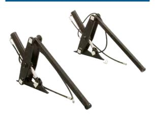
Fully hydraulic retrofit kits for front loader, tilt angle up to 180° / 850 mm stroke, tensile force per cylinder 3,450 daN at 180 bar, compression force per cylinder 2,300 daN at 180 bar, including hydraulic hoses.
