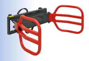
With Euro-bracket (125.024.600) and LP-bracket system (125.024.620) for front-, telescopic- or wheel loaders (please order adapter plates separately), for round bales, including hydraulic cylinder and hydraulic hoses with quick connector BG3.
