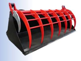
With LP-bracket for front-, telescopic- or wheel loaders (please order adapter plates separately), with hardened 500 HB cutting edge, protective runners at the bucket base, generously dimensioned hydraulic cylinders and hydraulic hoses with quick connector BG3.
