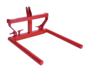
With Euro- and three-point bracket, mechanically adjustable in 50 mm increments, the steel support tubes (1,200 mm long) close with a round cap, adjustable for road transportation, optional with heavy duty tines.
