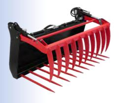
With LP-bracket for front-, telescopic- or wheel loaders (please order adapter plates separately) wear plate at the bottom, 900 mm forged tines, thickwalled side plates, hydraulic cylinders, hydraulic hoses, quick connector BG3.
