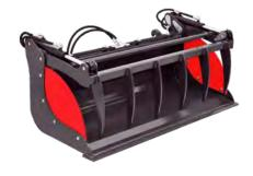
For small tractors, wheel and compact loaders (645 mm high), with Euroor LP mini-bracket, the bucket metal is 6 mm thick, two side panels, hydraulic cylinder and hydraulic hoses with quick connector BG3, cutting edge of hardened steel 500 HB, maximum opening width of 1,050 mm.
