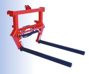
With Euro- and three-point bracket, the hydraulic bale handler with hydraulic cylinder and hydraulic hoses with quick connector BG3, the heavy duty forged steel tines are covered with demountable pivoting steel tubes to protect the bale wrap.
