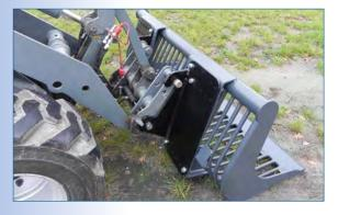
The punched plates (LP) bracket can be used to connect all common front loaders, wheel loaders, telescopic- or compact loaders to ourm devices.
