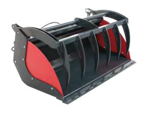
With LP-bracket for front-, telescopic- or wheel loaders (please order adapter plates separately), bucket metal 8 mm thick, incl. side plates, hydraulic cylinders and hydraulic hoses with quick connector BG3, double wear resis-tant 500 HB cutting edge, protective runners at the bucket base, 1,100 mm high.
