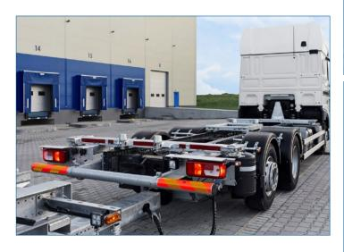
The pre-assembled Schneider BDF systems are simply bolted together. The same vehicle can transport containers of different lengths by means of double locks and/or the folding front stop.
