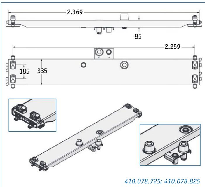
For transporting different container lengths flush with the cab, these are equipped **with double twist locks**. This is particularly important for vehicle combinations with center axle or turntable trailers.
