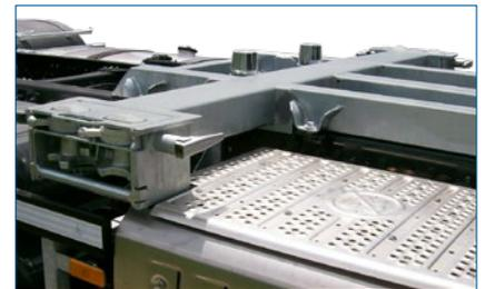
Schneider BDF bolsters cover the usual container lengths and **up to 3 parking levels of 1,020 - 1,220 mm or 1,120 - 1,320 mm**. On request, they are available with integrated or welded-on guide rollers.
