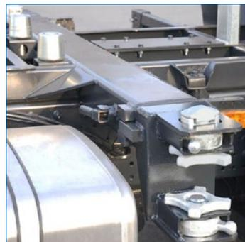
The **height-adjustable swap body bolster** include **three lift-lock types** as well as **countless swivelling variations**, which we configure for you, tailored to the application.
