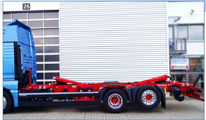
In the range of **rigid bolsters** with single or double twist locks, **the bolster 410.077.700** is a **new addition** for transporting different container lengths flush with the cab:
