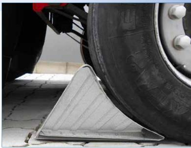
The supports with different internal widths for the various drag shoe sizes are also protected against corrosion by hot-dip galvanising.
