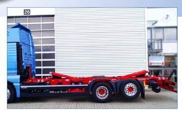
In the range of **rigid bolsters** with single or double twist locks, **the bolster 410.077.700 is a new addition** for transporting different container lengths flush with the cab:
