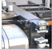
The height-adjustable swap body bolster include three lift-lock types as well as countless swivelling variations, which we configure for you, tailored to the application.
