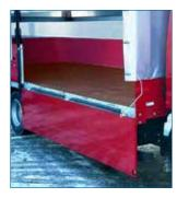
We manufacture and supply the drop sides to your specification in all standard RAL colours. The strong profiles can withstand heavy loads. They can be used with one pair of centre stanchions in conjunctions for loads up to 13 tonnes and up to 18 tonnes with two pairs of stakes.
