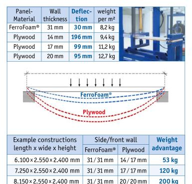
FerroFoam<sup>®</sup> panels are lighter than plywood walls, and their deflection stiffness is significantly higher in each case.
