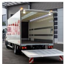
certificate for body stability / load securing in accordance with DIN EN 12642-XL.
