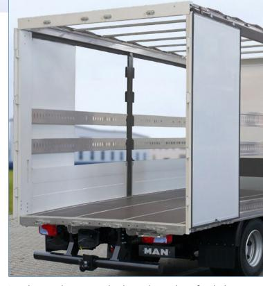
Last but not least, you also have the option of ordering the **kit with insert slats** in various designs as well as with a **dropside** including a groove for the tarpaulin.
