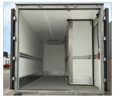
With the flush-mounted scuff rails of the FerroFoam® kits, you gain at least 12 mm interior width, with a longitudinal partition even 24 mm.
