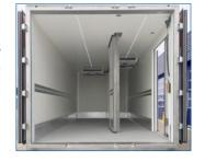
For individual customer installations you can order empty horizontal crimps. You can also get horizontal crimps with recessed snap in tracks, lashing rails or airline rails.
