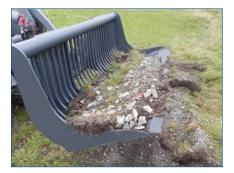
The device is also interesting for gardening and landscaping. It can be used to excavate paved paths easily and effectivel while at the same time recovering the old
