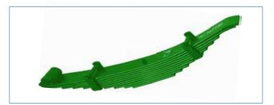
The **trapezoidal spring** is robust, cost effective and easy to repair. The individual layers of the spring are of equal strength throughout their length and are in contact with each other, resulting in **good inherent damping**.
