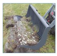
**The Sieve Bucket Mini** with 20 mm round rods at a distance of 40 mm removes stones from the soil, loads root crops cleanly, aerates topsoil, picks up wet soil, unpacks paving roads and much more.
