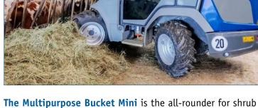
**The Multipurpose Bucket Mini** is the all-rounder for shrub cuttings, manure or other loose and bulky loads. The screwable side plates prevent loss of the load.
