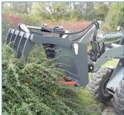
**The Fork With Grapple Mini** enables the removal and feeding of grass and corn silage as well as the transport of manure, straw, green waste and shrub cuttings. **The opening width of 822 mm is an absolute plus.** The wear plate under the lower protected tines ensures a long service life.
