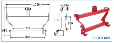
The lockable lower three-point brackets and the adjustable upper three-point brackets ensure
