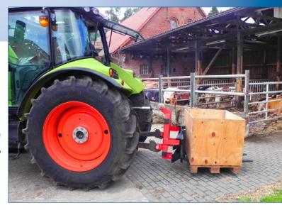
The **Schneider Euro adapter** made of higher strength steel offers the possibility to effectively drive existing devices with Cat. 2 three-point intake on the front loader with Euro bracket.
