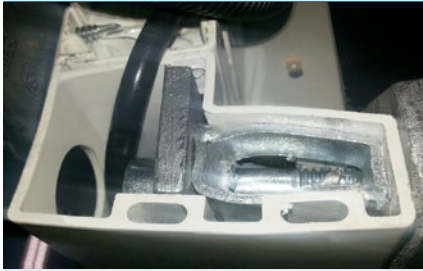
tightening torque too high
