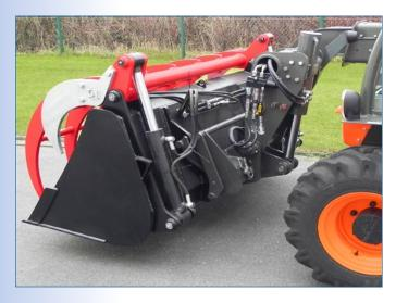
Due to pressure pulses, wear, ageing, damage, defective connection etc. hydraulic hoses represent a special hazard. Therefore operators of machines must check the hose lines prior to first use and after that at regular intervals, and exchange them in the case of a fault and due to ageing. The hydraulic hoses / lines are to be changed after two years at the latest.
